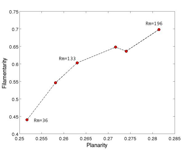
F/P grows with  $R_{\rm m}$ : magnetic filaments at  $R_{\rm m} \gg 1$ ;
