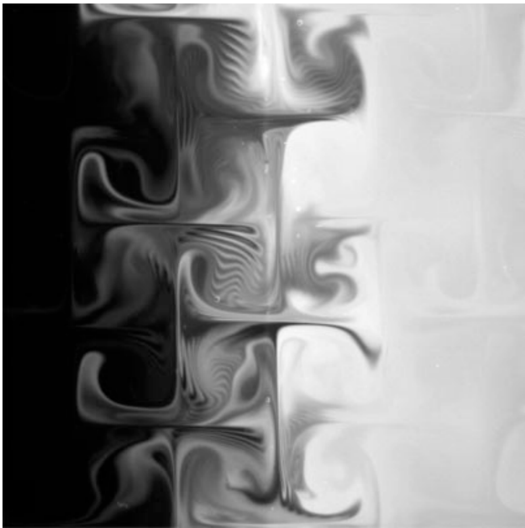
Figure 1 Snapshot of the concentration field for transient magnetically forced chaotic mixing. Fluid labelled with fluorescein was initially confined to the right half of the 20 \times 24 cm cell; the imaged region is 9.4 \times 9.4 cm. The light intensity under ultraviolet illumination is shown after 20 periods of forcing by a time periodic electric current at 100 mHz, in the presence of a spatially periodic magnet array. The repetitive stretching and folding that is characteristic of chaotic advection is evident.
