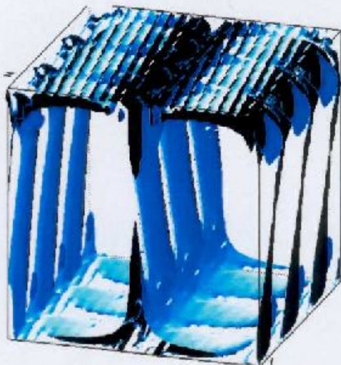
Figure 8: Growing magnetic field for the flow given by \psi , W_2 , with k = 1.5 , m = 1 and R = 2000 . An isosurface of constant magnetic field magnitude is shown in three dimensions.
